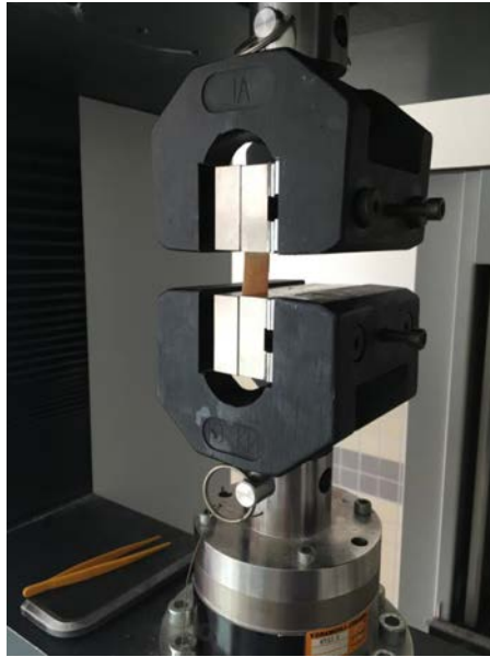
Fig. 3. MTS 20 M traction device and explanatory diagram of the traction system.
