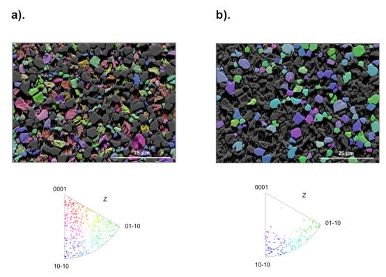
Fig. 3. Pure β-TCP acid-etched for 1 h: overlay of SEM images and crystal orientation maps derived from EBSD and displayed in Inverse Pole Figure (IPF) coloring (the reference direction is Z, i.e. the normal direction to the map): (a) etched grains and corresponding IPF (b) non-etched grains and corresponding IPF.
