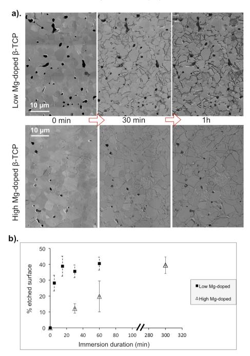
**Fig. 1.** a). SEM images of low Mg-doped and high Mg-doped β-TCP samples as-prepared ("0 min") and immersed for different durations in acidic solution; b) percentage of etched surface versus immersion time in acidic solution. In high-Mg-doped samples, etched and non-etched grains can hardly be discriminated before 30 min.
