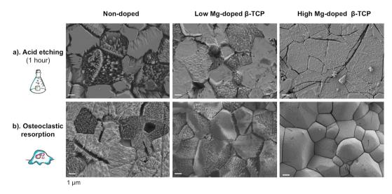
**Fig. 2.** SEM images of the surfaces of non-doped and Mg-doped β-TCP samples: a). after 1 h immersion in the acidic solution (above) and b). after 24 h of contact with osteoclast cells (RANKL concentration = 20 ng/mL, below). Scale bar =  $1 \mu m$  for all micrographs.
