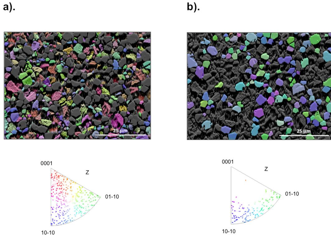
**Fig. 3.** Pure  $\beta$ -TCP acid-etched for 1 h: overlay of SEM images and crystal orientation maps derived from EBSD and displayed in Inverse Pole Figure (IPF) coloring (the reference direction is Z, i.e. the normal direction to the map): (a) etched grains and corresponding IPF (b) non-etched grains and corresponding IPF.
