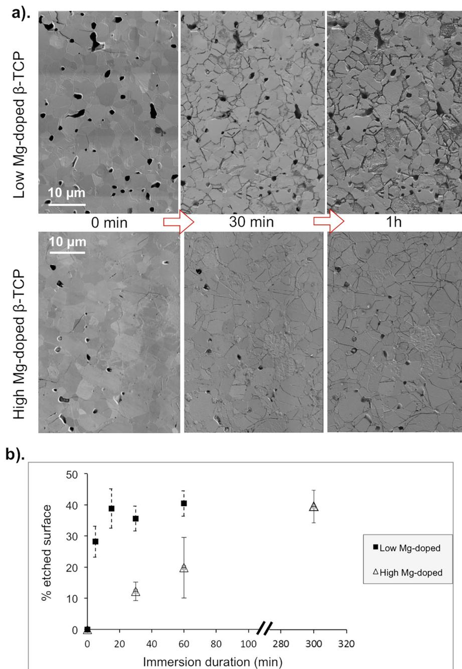
**Fig. 1.** a). SEM images of low Mg-doped and high Mg-doped  $\beta$ -TCP samples as-prepared (“0 min”) and immersed for different durations in acidic solution; b) percentage of etched surface versus immersion time in acidic solution. In high-Mg-doped samples, etched and non-etched grains can hardly be discriminated before 30 min.
