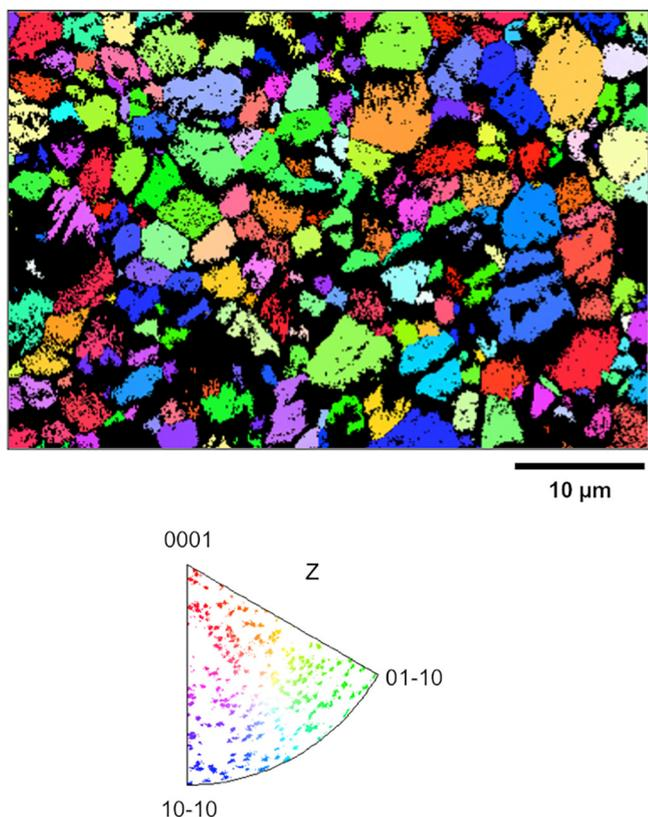
**Fig. 6.** Pure  $\beta$ -TCP after 24 h of contact with osteoclast cells (RANKL concentration = 5 ng/mL): overlay of a SEM image and crystal orientation maps derived from EBSD and displayed in Inverse Pole Figure (IPF) coloring (the reference direction is Z, i.e. the normal direction to the map).
