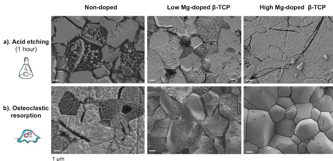
**Fig. 2.** SEM images of the surfaces of non-doped and Mg-doped  $\beta$ -TCP samples: a). after 1 h immersion in the acidic solution (above) and b). after 24 h of contact with osteoclast cells (RANKL concentration = 20 ng/mL, below). Scale bar = 1  $\mu\text{m}$  for all micrographs.
