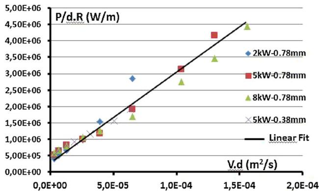
Fig. 1. For St35 steel and different operating parameters (incident powers and focal spot diameters), plot of  $P/(d.R)$  as a function of the parameter  $V.d$  and corresponding best linear fit (KH depths obtained by [Suder and Williams, \(2014\)](#) at  $1.06 \mu\text{m}$  laser wavelength).
