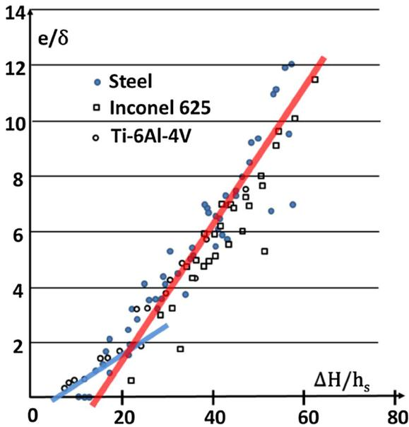
Fig. 2. Normalized melt pool depth  $e/\delta$  as a function of normalized enthalpy  $\Delta H/h_s$  (from Rubenchick et al., 2018 and King et al., 2014). The data for the conduction regime have been fitted with the blue line and those for the KH regime with the red one (For interpretation of the references to colour in this figure legend, the reader is referred to the web version of this article).
