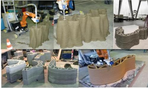
Figure 9. FABRICATION ADDITIVE AVEC LE ROBOT MATRICE
