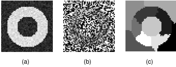
Fig. 1. Example illustrating that K-Means does not preserve connectivity. (a) Example grey scale image. (b) Clusters obtained using K-Means on the greyscale values of (a). (c) Clusters obtained using adapted K-Means algorithm as proposed in this article. This figure is also shown in [4].
