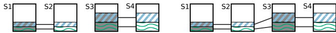
(a) In dedicated protection each slave protects at most one master. In this example each master has a single slave.
