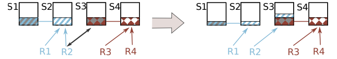
Figure 9: Example of request move neighborhood: request R_2 is moved and assigned to a different server.
