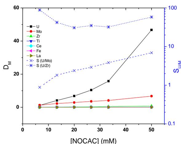
Figure 11: Effect of the concentration of NOCAC on the distribution values and selectivities,  $S_{(U/M)}$ . Organic phase: NOCAC 0.01–0.05 M in dodecane/octanol (83/17 v/v). Aqueous phase: 25 ppm of each metal in 0.1 M  $H_2SO_4$ .
