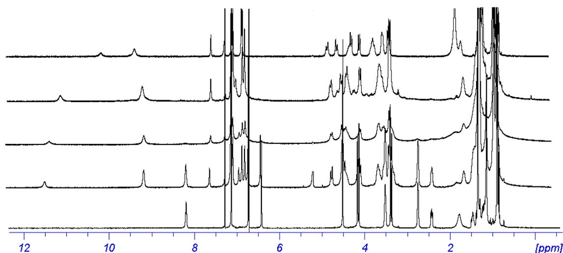
Figure 7: NMR titration spectra of the ligand NOCAC with  $\text{UO}_2(\text{NO}_3)_2$  at different ratios varied from  $[\text{NOCAC}]/[\text{UO}_2^{2+}] = 1:0$  to  $1:2$ ,  $[\text{NOCAC}] = 30$  mM in  $\text{CDCl}_3$ .
