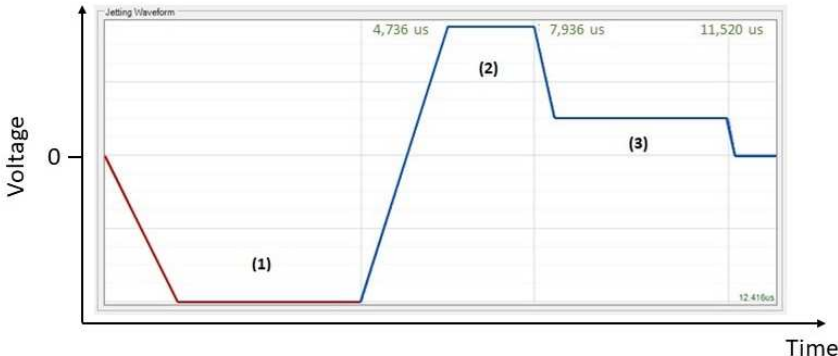
Figure 2. Electric pulse generating \text{TiS}_2[(\text{HA})_x(\text{NMF})_y] drops.
