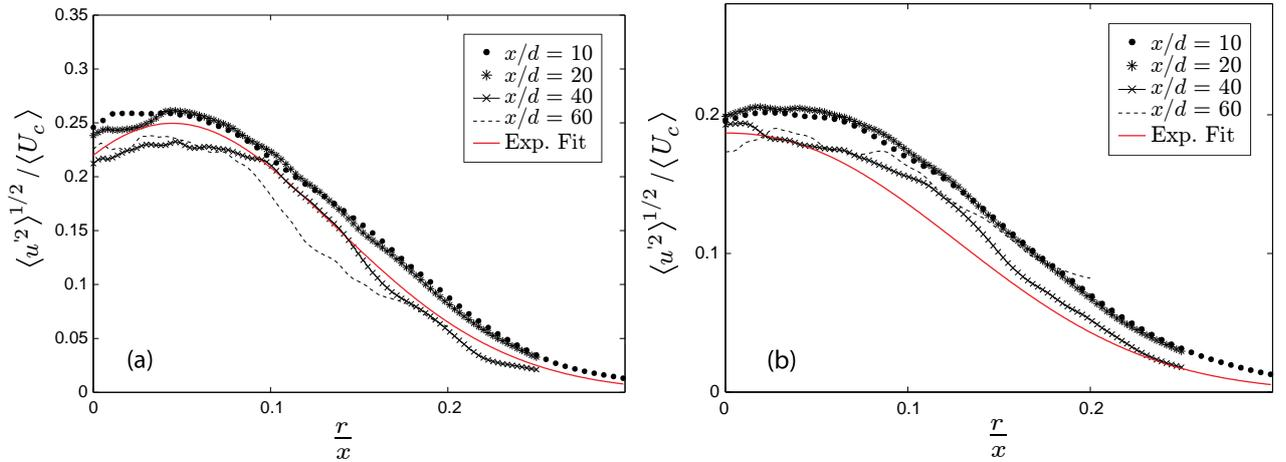
Figure 6: Radial profiles of the rms of the axial velocity,  $\sqrt{\langle u'^2 \rangle}$  (a), and the radial velocity  $\sqrt{\langle v'^2 \rangle}$  (b), normalised by the mean centerline velocity  $\langle U_c \rangle$  for the jet  $H_2$
