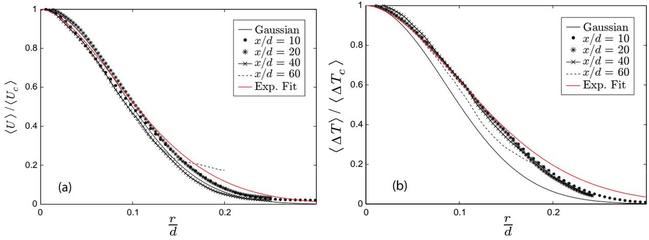
Figure 4: Radial profiles of mean axial velocity normalised by the mean centerline velocity  $\langle U_c \rangle$  (a) and mean radial temperature variation  $\langle \Delta T \rangle = \langle T - T_0 \rangle$  normalised by the mean centerline temperature variation  $\langle \Delta T_c \rangle = \langle T_c - T_0 \rangle$  (b)
