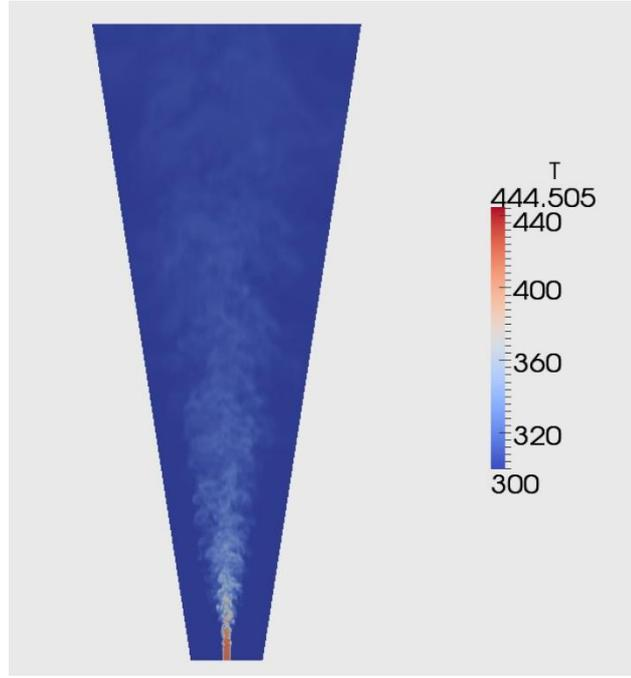
Figure 1: Example of instantaneous temperature field (in  $K$ ) of the jet  $H_1$  in a plane  $(x, r)$ .
