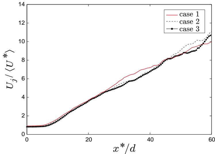
Figure 7: Centerline velocity decay using the scaling law proposed by Chen and Rodi [1980], *i.e.*,  $x^* = s^{-1/4}x$  and  $\langle U^* \rangle = s^{-1/4}\langle U_c \rangle$  with  $s = \rho_j / \rho_0$
