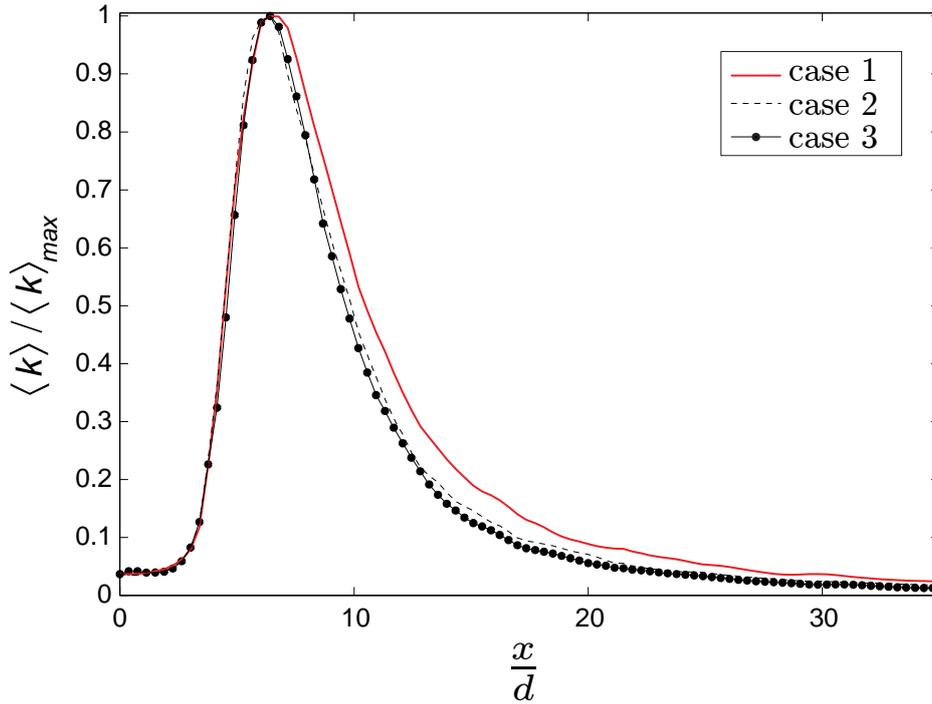
Figure 8: Mean turbulent kinetic energy  $\langle k \rangle$  normalised by the maximum value  $k_{\max}$  along the centerline for the three jets
