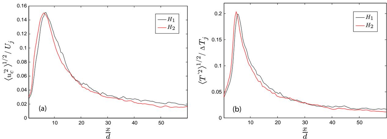
Figure 5: rms of the axial velocity component at the centerline  $\sqrt{\langle u_c^2 \rangle}$  normalised by the jet velocity,  $U_j$  (a) and rms of the temperature at the centerline  $\sqrt{\langle T_c^2 \rangle}$  normalised by the jet temperature variation  $\Delta T_j$  for the two jets (b)
