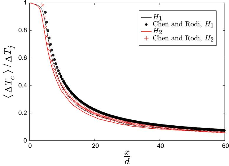
Figure 3: Mean centerline temperature variation  $\langle \Delta T_c \rangle$  normalised by the difference between the jet temperature at the exit of the nozzle,  $T_j$ , and the ambient temperature,  $T_0$ .
