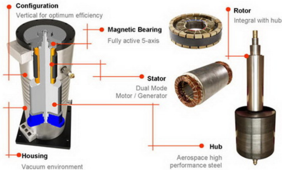
Exemple de structure industrielle – MSAP - 300kW/800 Wh http://www.vyconenergy.com/pages/flywheeltech.htm
