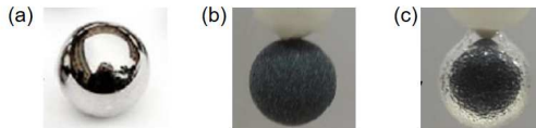
FIGURE 3. Images taken during the manufacturing procedure of a d = 10 mm SH sphere illustrating: (a) reference stainless steel sphere, (b) intermediate layer made of a carbon-based powder, (c) air plastron around the surface of the SH sphere once immersed in water.
