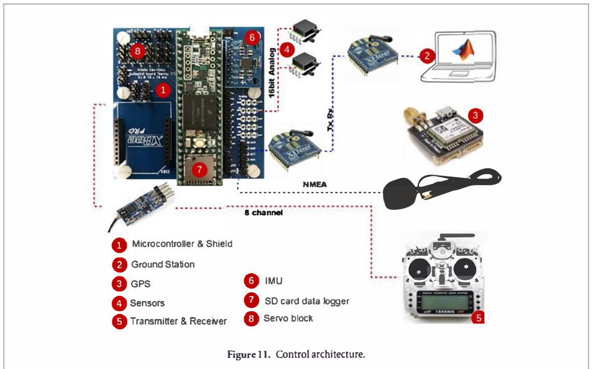
Figure 11. Control architecture.
