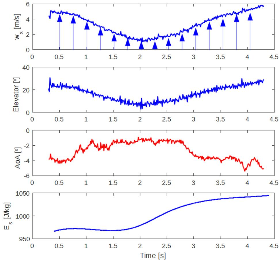
Figure 21. Energy-harvesting within horizontal wind velocity gradient.
