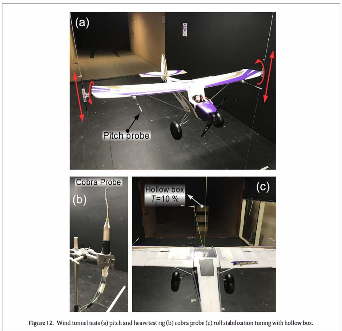
Figure 12. Wind tunnel tests (a) pitch and heave test rig (b) cobra probe (c) roll stabilization tuning with hollow box.
