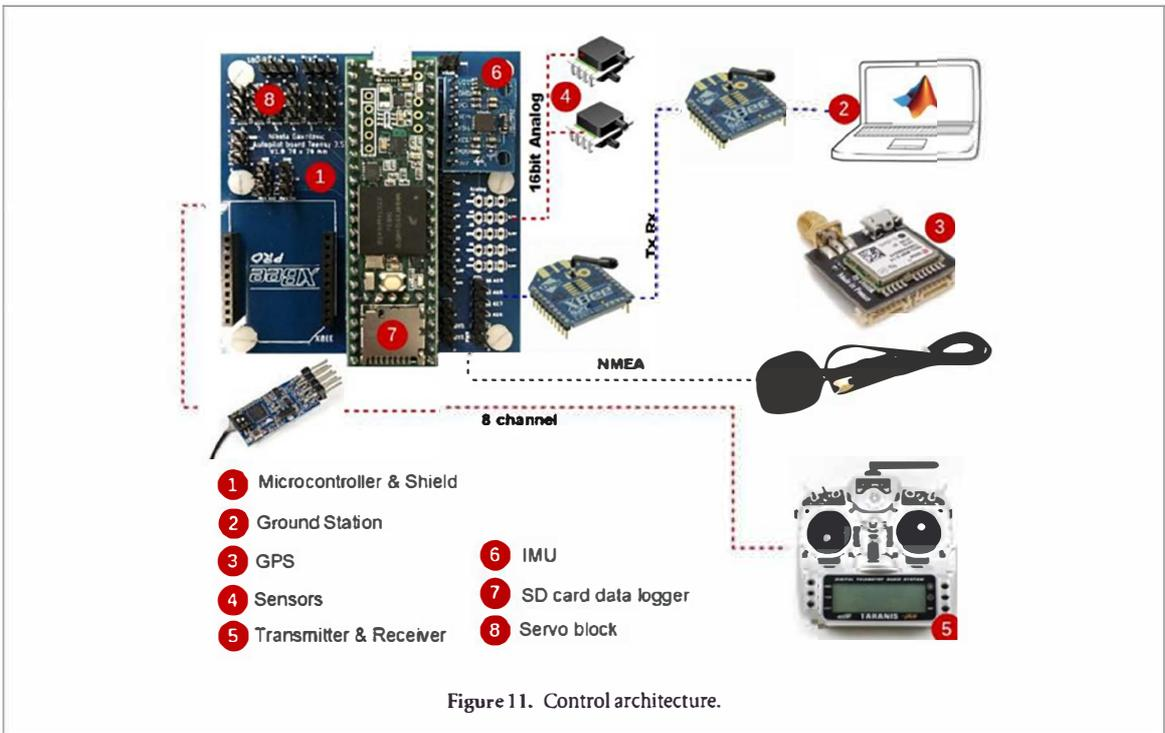
Figure 11. Control architecture.
