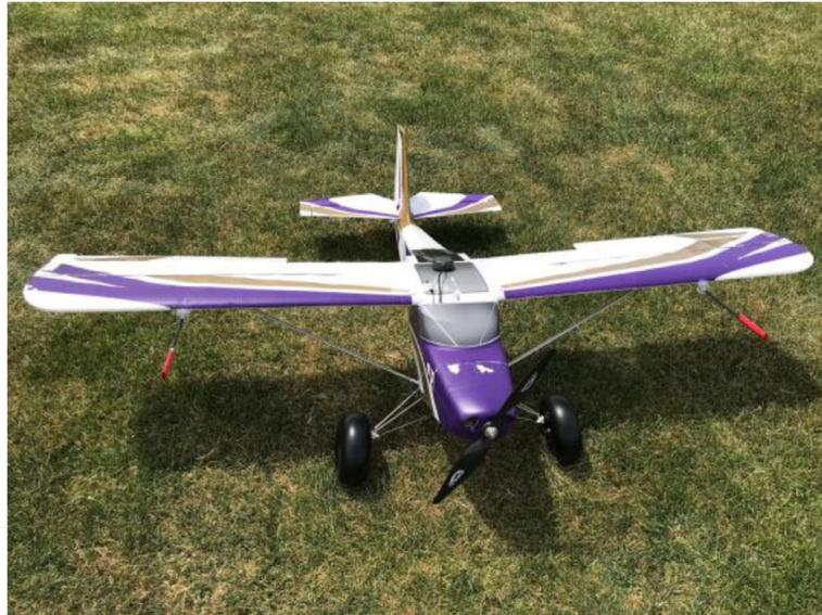
Figure 10. MAV airframe with pitch probes.
