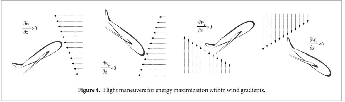
Figure 4. Flight maneuvers for energy maximization within wind gradients.
