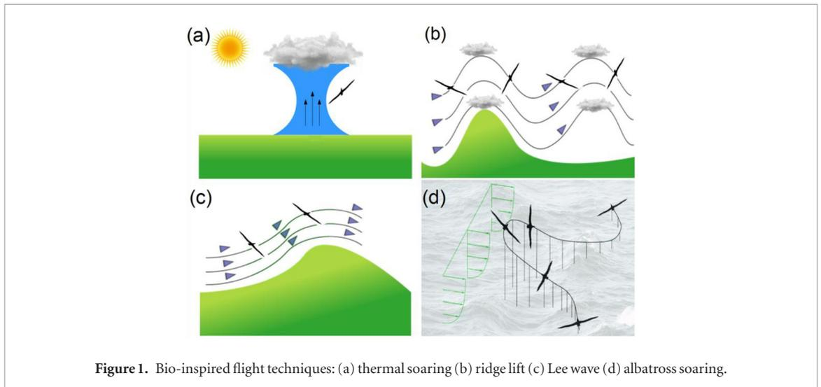
**Figure 1.** Bio-inspired flight techniques: (a) thermal soaring (b) ridge lift (c) Lee wave (d) albatross soaring.
