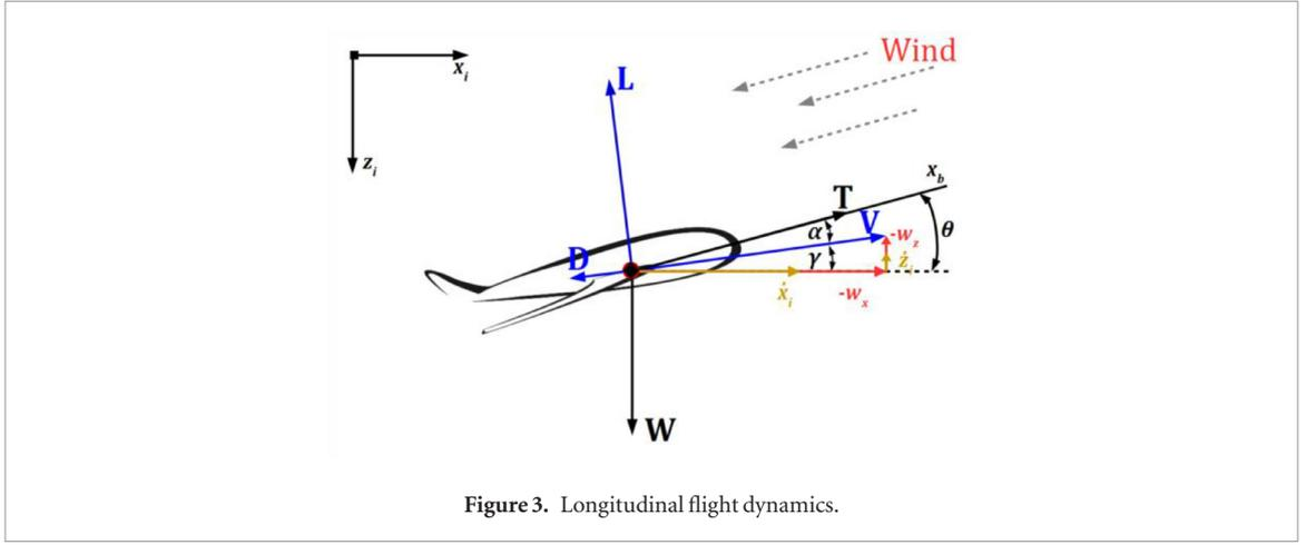
Figure 3. Longitudinal flight dynamics.
