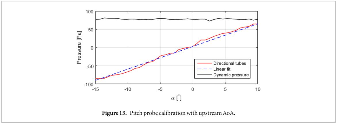
Figure 13. Pitch probe calibration with upstream AoA.
