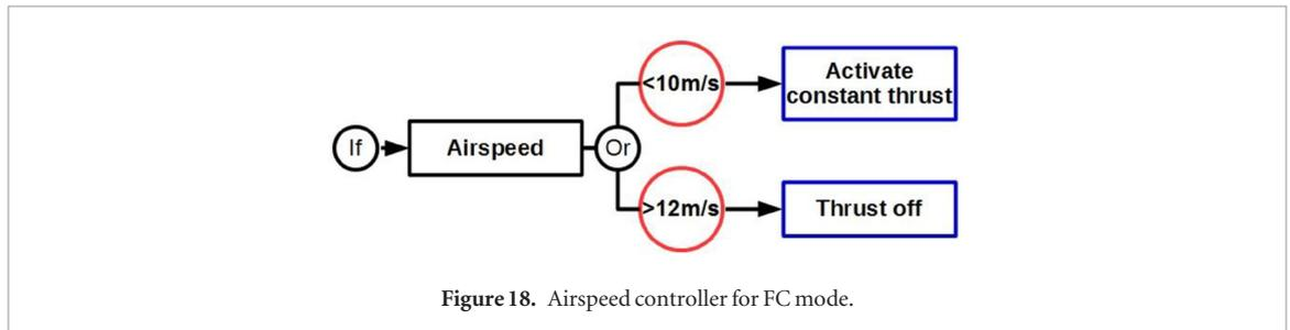
Figure 18. Airspeed controller for FC mode.
