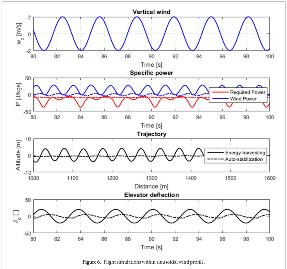
Figure 6. Flight simulations within sinusoidal wind profile.
