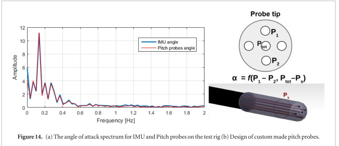
Figure 14. (a) The angle of attack spectrum for IMU and Pitch probes on the test rig (b) Design of custom made pitch probes.
