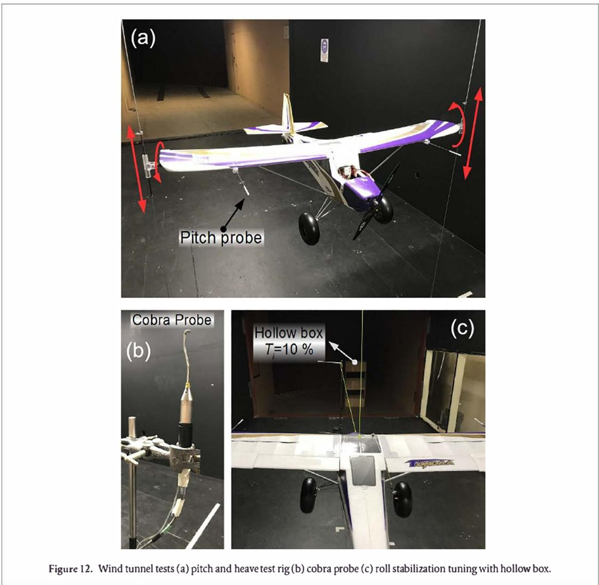
Figure 12. Wind tunnel tests (a) pitch and heave test rig (b) cobra probe (c) roll stabilization tuning with hollow box.
