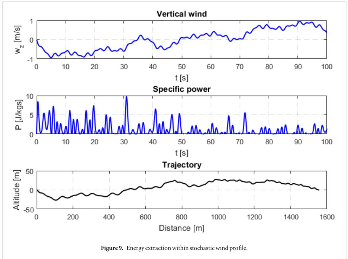
Figure 9. Energy extraction within stochastic wind profile.
