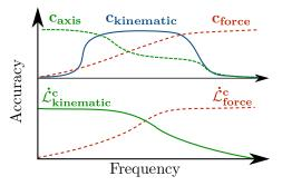
Fig. 2: Schematic representation of the spectral accuracy of the different input signals for the estimation of c and  $\dot{\mathcal{L}}^{c}$ .
