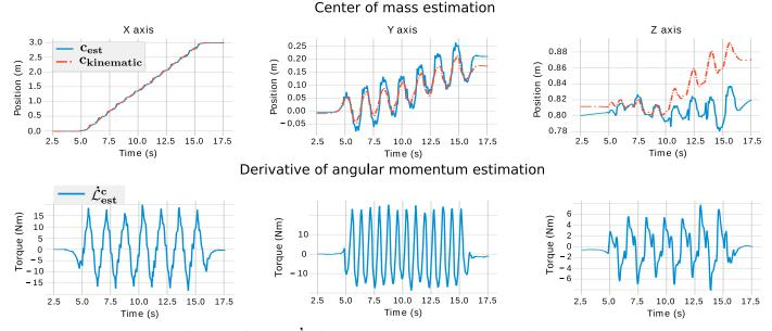
Fig. 9: *Experimentation*. Estimation of **c** and  $\dot{\mathcal{L}}^{c}$  for a horizontal walking motion of the HRP-2 robot. First row  $\mathbf{c}_{est}$  and  $\mathbf{c}_{kinematic}$ . Second row :  $\dot{\mathcal{L}}_{est}^{c}$ .
