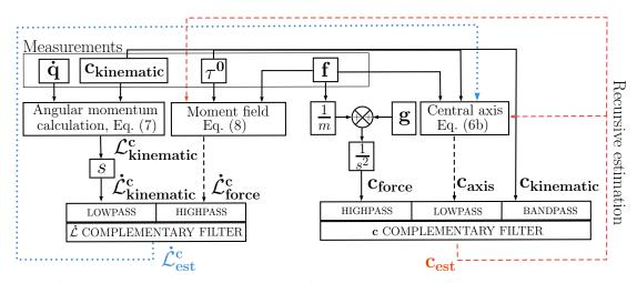
Fig. 3: Flow chart of the recursive complementary estimation framework, with s the Laplace variable. Dotted lines represent the update step of the algorithm. Complementary filtered components are summed in order to output  $\dot{\mathcal{L}}_{est}^{c}$  and  $\mathbf{c}_{est}$ , the estimates of  $\dot{\mathcal{L}}^{c}$  and  $\mathbf{c}$  respectively.
