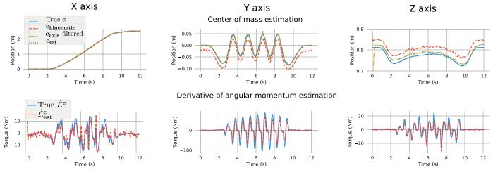
Fig. 7: *Simulation*. Estimation of **c** and  $\dot{\mathcal{L}}^{\mathbf{c}}$  for a horizontal walking motion of the HRP-2 robot in simulation. First row : true **c**,  $\mathbf{c}_{kinematic}$ ,  $\mathbf{c}_{axis}$  and  $\mathbf{c}_{est}$ . Second row :  $\dot{\mathcal{L}}_{est}^{\mathbf{c}}$  and true  $\dot{\mathcal{L}}^{\mathbf{c}}$ .
