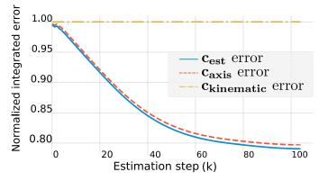
Fig. 4: *Simulation*. Evolution of the error 2-norm integrated over the whole trajectory for  $c_{kinematic}$ ,  $c_{axis}$  and  $c_{est}$ . This plot is the result of the algorithm in Fig. 5. The integrated errors are normalized with regard to the error of  $c_{kinematic}$ , which is the initialization of the algorithm and is not updated throughout the iterations (and therefore constantly 1.)
