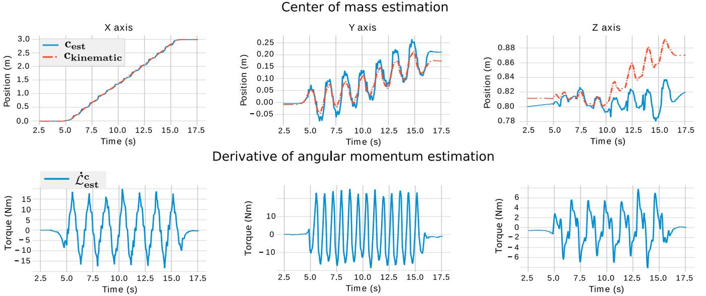
Fig. 9: *Experimentation*. Estimation of  $\mathbf{c}$  and  $\dot{\mathbf{L}}^c$  for a horizontal walking motion of the HRP-2 robot. First row  $\mathbf{c}_{est}$  and  $\mathbf{c}_{kinematic}$ . Second row :  $\dot{\mathbf{L}}^c_{est}$ .
