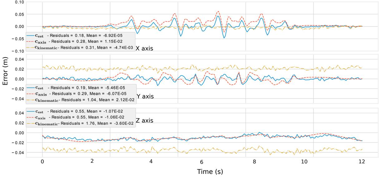
Fig. 6: *Simulation*. Time residuals of  $c_{kinematic}$ ,  $c_{axis}$  and  $c_{est}$  after convergence of the recursive algorithm, for a horizontal walking motion of the HRP-2 robot in simulation. The 1-norm and the mean of the residuals are displayed.
