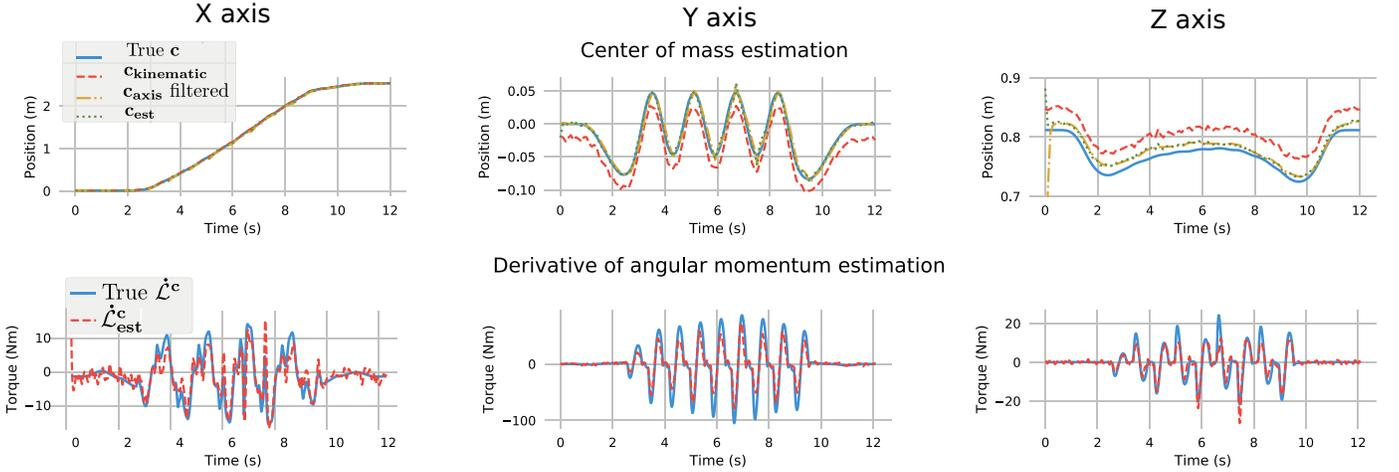
Fig. 7: *Simulation*. Estimation of  $c$  and  $\dot{L}^c$  for a horizontal walking motion of the HRP-2 robot in simulation. First row : true  $c$ ,  $c_{kinematic}$ ,  $c_{axis}$  and  $c_{est}$ . Second row :  $\dot{L}^c_{est}$  and true  $\dot{L}^c$ .
