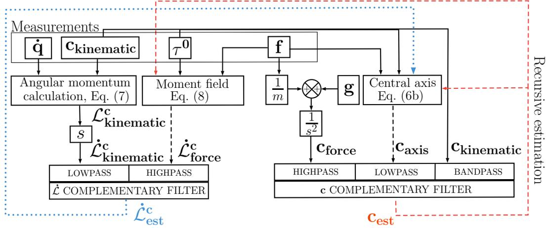
Fig. 3: Flow chart of the recursive complementary estimation framework, with  $s$  the Laplace variable. Dotted lines represent the update step of the algorithm. Complementary filtered components are summed in order to output  $\hat{L}^c_{est}$  and  $c_{est}$ , the estimates of  $\dot{L}^c$  and  $c$  respectively.
