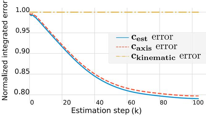
Fig. 4: *Simulation*. Evolution of the error 2-norm integrated over the whole trajectory for  $\mathbf{c}_{\text{kinematic}}$ ,  $\mathbf{c}_{\text{axis}}$  and  $\mathbf{c}_{\text{est}}$ . This plot is the result of the algorithm in Fig. 5. The integrated errors are normalized with regard to the error of  $\mathbf{c}_{\text{kinematic}}$ , which is the initialization of the algorithm and is not updated throughout the iterations (and therefore constantly 1.)
