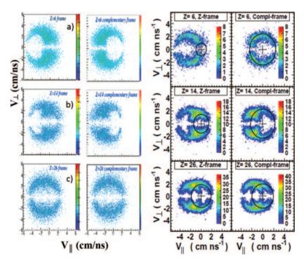
Fig. 6.  $-v_{\perp}$  vs.  $v_{\parallel}$  plot for the n-poor system, in the frame of the light fragment and in its complementary partner's frame, on the left for incident energy  $E=10\,\mathrm{A\,MeV}$  and on the right for  $E=5.5\,\mathrm{A\,MeV}$ .
