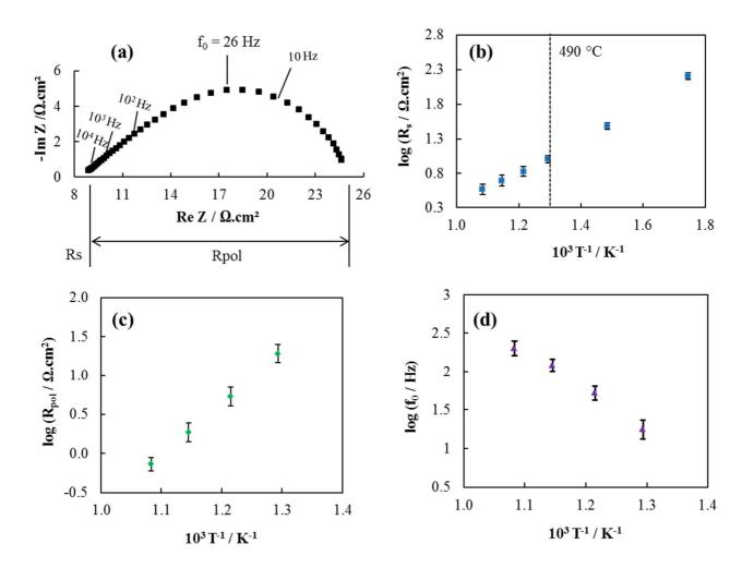
Fig.2. (a) Typical impedance spectrum at OCV ( $pO_2 = 0.21$  atm, T = 500 °C). Arrhenius plot of (b) R<sub>s</sub>, (c) R<sub>pol</sub> and (d) f<sub>0</sub>. The error was estimated from 4 similar porous films deposited on GDC.
