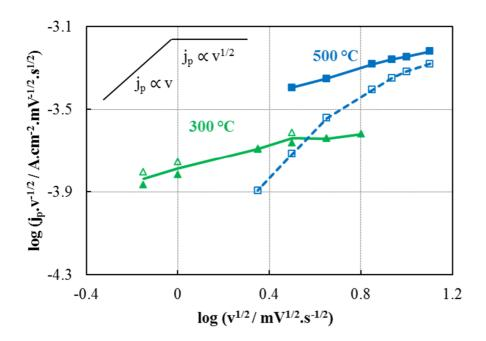
Fig. 7. Variation of the voltammetry parameters as a function of the scan rate for the dense film under  $pO_2 = 0.21$  atm.  $j_{pc}$  (filled symbol) and  $j_{pa}$  (empty symbol) at 300 °C (green) and 500 °C (blue). The line is only a guide for the eyes. The representation mode is the one proposed by Diard et al. [38].
