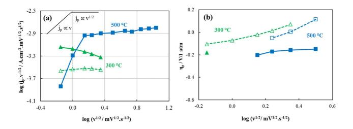
Fig. 9. Variation of the voltammetry parameters as a function of the scan rate for the porous film under  $pO_2 = 1.8 \times 10^{-4}$  atm. (a)  $j_{pc}$  (filled symbol) and  $j_{pa}$  (empty symbol) at 300 °C (green) and  $j_{pc}$  at 500 °C (blue). The line is only a guide for the eyes. (b)  $\eta_{pa}$  (empty symbol) and  $\eta_{pc}$  (filled symbol) at 300 °C (green) and at 500 °C (blue). The representation mode is the one proposed by Diard et al. [38].
