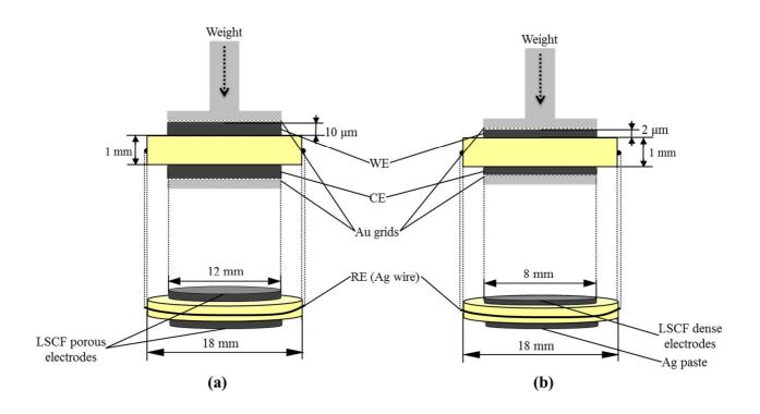
Fig.1. Description of the three-electrode set-up. Cell dimensions and nature of the electrodes for tests with porous LSCF (a) and dense LSCF (b).
