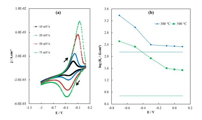
Fig. 5. Typical electrochemical measurements for the dense LSCF electrode under  $pO_2 = 0.21$  atm. (a) Cyclic voltammetry (pre-treatment 0.1 V for 600 s, T = 500 °C). (b) R<sub>s</sub> dependence on applied dc potential (E). For comparison Rs<sup>GDC</sup> calculated from Steele's data [29] at 300 °C and 500 °C is represented by the dashed lines.
