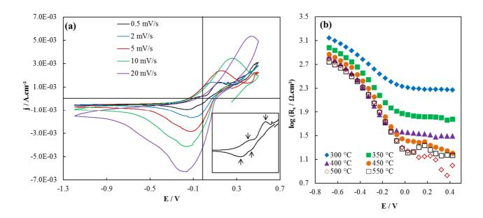
Fig. 8. Typical electrochemical measurements for the porous LSCF electrode under  $pO_2 = 1.8 \times 10^{-4}$  atm. (a) Cyclic voltammetry (pre-treatment 0.25 V for 600 s, T = 500°C). The insert shows a zoom of the voltammetry curve at 0.5 mV.s<sup>-1</sup>. (b) R<sub>s</sub> dependence on applied dc potential (E) for different temperatures.
