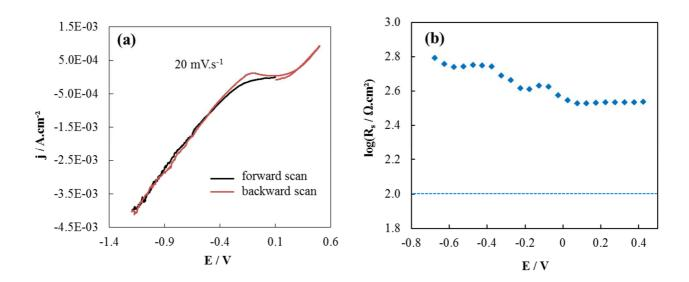
Fig. 11. Electrochemical measurements for the columnar LSCF electrode under  $pO_2 = 0.21$  atm at T= 300°C. (a) Cyclic voltammetry (pre-treatment 0.1 V for 600 s). (b) R<sub>s</sub> dependence on applied dc potential (E). For comparison R<sub>s</sub><sup>GDC</sup> calculated from Steele's data [29] is represented by the dashed line.
