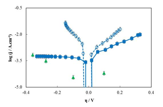
Fig. 10. Comparison of the polarization curves of the porous thick film (blue) under  $pO_2 = 0.21$  atm (empty symbol) and  $pO_2 = 1.8 \times 10^{-4}$  atm (filled symbol) at 500 °C. A few points corresponding to the log (j) *vs*  $\eta$  curve for the dense thin film (green) are indicated (T = 500 °C,  $pO_2 = 0.21$  atm).
