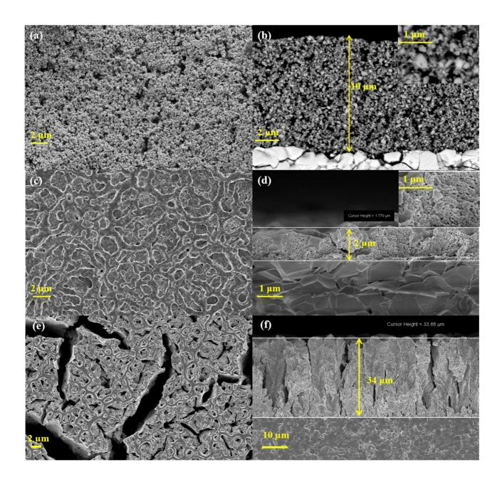
Fig.3. SEM images of the surface (on the left) and the cross-section (on the right) for the different LSCF electrodes. (a) and (b) SP porous sample. (c) and (d) ESD almost dense sample. (e) and (f) ESD columnar sample
