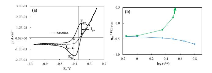
Fig. 6. (a) Peak current and peak potential determination mode. (b) Peak potential,  $\eta_p$ , determined according to Eq. (1) with  $R_s = R_s(OCV)$  (blue) or  $R_s = R_s(E)$  (green). The determination mode is illustrated on the cathodic peak at 300 °C. The green arrow indicates a large increase in  $\eta_{pc}$ .
