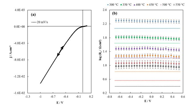
Fig. 4. Typical electrochemical measurements for the porous LSCF electrode under  $pO_2 = 0.21$  atm. (a) Cyclic voltammetry (pre-treatment 0.1 V for 600 s, T = 407 °C). (b) R<sub>s</sub> dependence on applied dc potential (E) for different temperatures. For comparison R<sub>s</sub><sup>GDC</sup> calculated from Steele's data [29] at the same temperatures is represented by the dashed lines.
