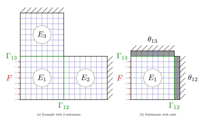
Figure 3: Example of a subdomain with its soles
