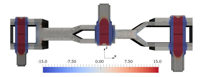
Figure 11: Preload of bolts - stress  $\sigma_{zz}$  (MPa)
