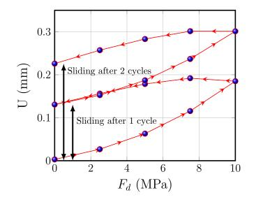
Figure 13: Mean longitudinal displacement at the end of the structure
