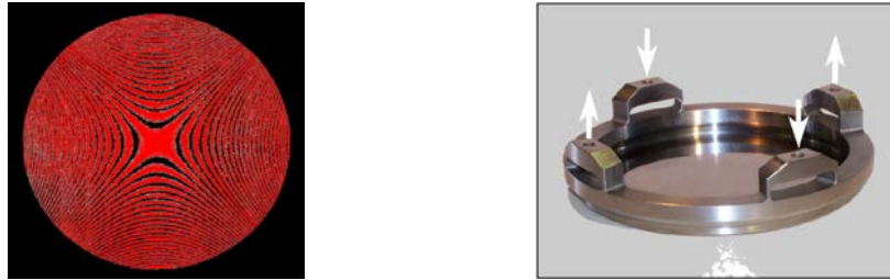
Fig. 4. Left : Cycloid-like deformable submaster generating A_{22} mode from four forces. Thickness distributions t/t_0 = (1 - \rho^2)^{1/3} . Right : He-Ne fringes of a first replica grating on active submaster for obtaining by replication one of the toroid A_{22} -corrected grating replicas of spectrographs UVCS and CDS of SOHO Mission (LOOM, ETH-Zurich, Bach Research Corp-Boulder).
