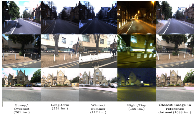
Fig. 3. Examples of test images : we evaluate our proposal on four challenging localization sequences. The number under the query set name indicates the amount of query images to compare against the 1688 reference images.
