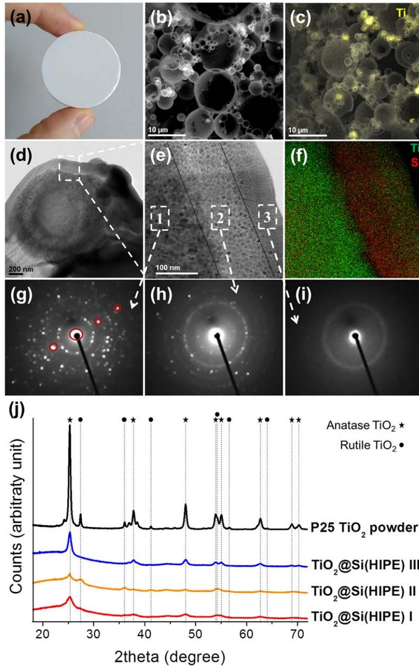
**Figure 1.** Multi-scale characterizations of  $\text{TiO}_2@Si(\text{HIPE})$  monoliths and crystalline structure of commercial reference  $\text{TiO}_2$  (P25  $\text{TiO}_2$  Degussa). **(a)** Photograph of a typical  $\text{TiO}_2@Si(\text{HIPE})$ . **(b)** SEM image of a typical  $\text{TiO}_2@Si(\text{HIPE})$ , at 15 kV, where  $\text{TiO}_2$  particles appear brighter. **(c)** SEM-EDS mapping of a typical  $\text{TiO}_2@Si(\text{HIPE})$  where titanium element is highlighted in yellow.
