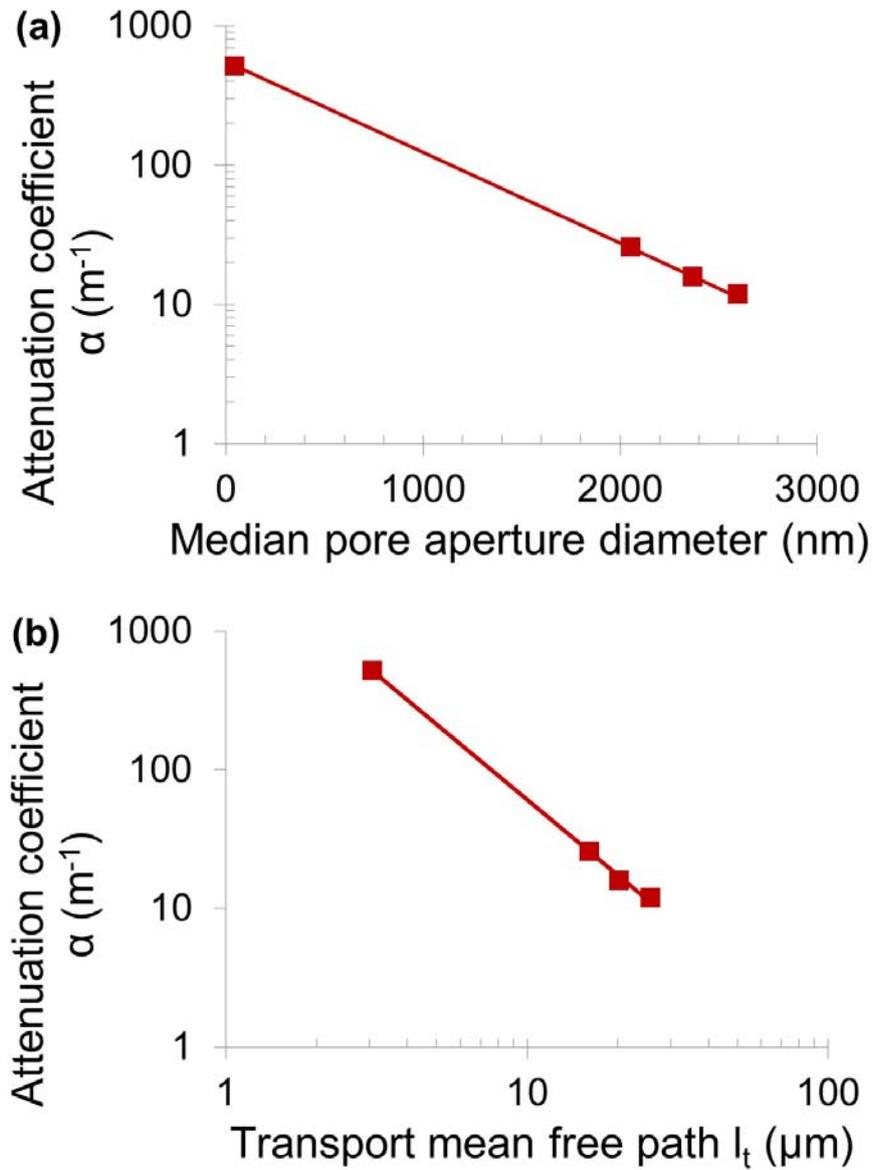
5 **Fig. 6.** Comparison between photonic and textural properties. Beer-Lambert attenuation
