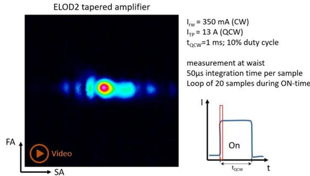
Video 1. A label of the video “spatial\_dynamics\_QCW.mp4”. The video was assembled out of beam shape measurements triggered on the QCW pulses. Each sample was recorded with 50  $\mu$ s integration time during the on-time  $\tau_{QCW}$  of 1 ms. The video therefore represents the spatial dynamics of the beam at the start of each pulse. The measurement plane was chosen at the waist of the stabilized beam at the end of each pulse. Link to the video: <http://dx.doi.org/doi.number.goes.here>.
