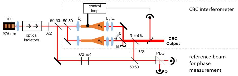
Figure 8. Experimental setup of the CBC-Interferometer and for phase measurements. PBS; Polarizing beam splitter; L1:  $f = 8$  mm,  $NA = 0.5$ ; L2:  $f = 8$  mm,  $NA = 0.5$ . L3:  $f = 2.75$ ,  $NA = 0.55$ , L4:  $f = 19$  mm. We used a triple stage faraday isolator with an optical isolation better than  $-72$  dB.
