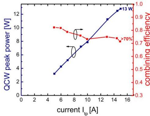
Figure 10. Power (QCW peak power) and combining efficiency at the output of the CBC interferometer for two ELOD2 tapered amplifiers.  $\tau_{\text{QCW}} = 5$  ms, 10 % duty cycle, heatsink  $T = 20^\circ\text{C}$ ,  $P_{\text{in}} = 15$  mW per amplifier.
