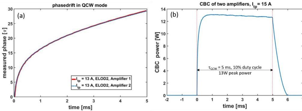
Figure 9. (a) Phase measurements for two ELOD2 amplifiers in QCW mode. (b) Photodiode measurement of the coherently combined beam from two ELOD2 amplifiers.  $300 \text{ mA} < I_{rw} < 400 \text{ mA}$  (CW, used for phase piston control),  $I_{tp} = 13 \text{ A}$  (QCW),  $\tau_{QCW} = 5$  ms, 10 % duty cycle, heatsink  $T = 20^\circ\text{C}$ ,  $P_{in} = 15 \text{ mW}$  per amplifier.
