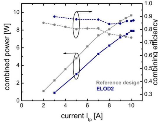
Figure 7. Power and combining efficiency for two amplifiers with the ELOD2 (blue) and with the reference design (red) in CW for different currents into the tapered section ( $I_p$ ). The injected seed power was 15 mW for all amplifiers and the heatsink temperature was 20°C.
