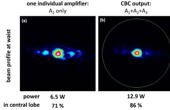
Figure 2. Beam profiles at waist for (a) one individual amplifier (reference design) and (b) the CBC output  $A_{1+2+3}$ . Measurement for  $I_{tp} = 10$  A,  $T = 20$  °C and actively controlled ridge currents in the range of 250 to 400 mA. The FA is in vertical and the SA is in horizontal direction. The given central lobe power content was calculated by fitting a Gaussian beam profile to the central lobe of the beam and calculating the power content within the fitted profile<sup>10</sup>.
