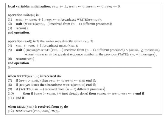
Figure 1: Time-efficient SWMR atomic register in  $\mathcal{AMP}_{n,t}[t < n/2]$
