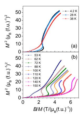
**Fig. 4:** Arrott-Belov curves of the  $Y_{0.5}Er_{0.5}Fe_2D_{4.0}$  S2 compound measured under high magnetic field (35 T) between 4.2 and 38 K (a) and 53 K to 150 K (b).
