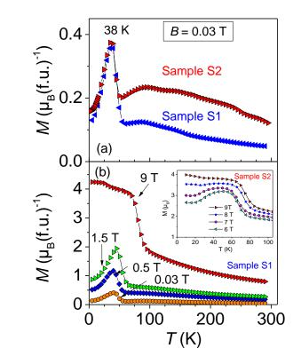
**Fig. 2** : Thermomagnetization curves of the  $Y_{0.5}Er_{0.5}FeD_4$  samples under different applied magnetic fields: a) comparison of S1 and S2 under 0.03T; b) Evolution of the magnetization curves under different applied field for sample S1 in main part and sample S2 in Inset.
