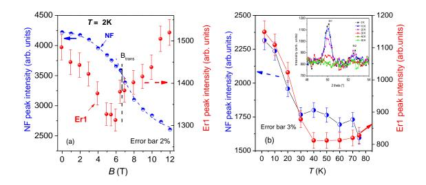
**Fig 12**: Variations of the NF and Er1 peak intensities of the  $Y_{0.5}Er_{0.5}Fe_2D_{4.2}$  deuteride versus applied magnetic field at 2K (a) and versus temperature under 10 T (b). The inset of Fig 12(a) corresponds to a zoom on Er1 and Er2 peaks at selected temperatures.
