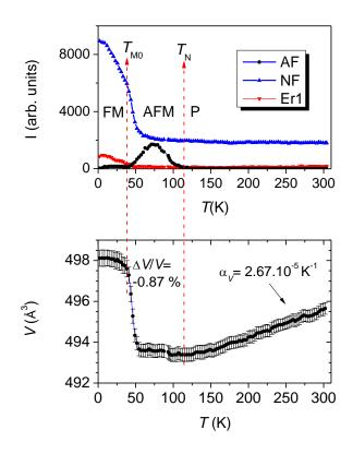
**Fig. 9:** Temperature dependence of (top) the intensities of AF, NF and Er1 Bragg peaks and (bottom) cell volume of  $Y_{0.5}Er_{0.5}Fe_2D_{4.2}$  in zero applied field for the S2 sample.  $T_{M0}$  and  $T_N$  positions are marked with dotted line as guide for eyes.
