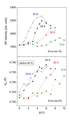
**Fig. 13:** Evolution of the NF peak intensity (top) and of the interplanar  $d_{\rm NF}$  distance (bottom) for Y<sub>0.5</sub>Er<sub>0.5</sub>Fe<sub>2</sub> D<sub>4.2</sub> deuteride at 50, 55, 65 and 75 K.
