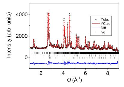
**Fig. 1**: Refined NPD pattern of  $Y_{0.5}Er_{0.5}Fe_2D_{4.2}$  (sample S2) measured in 3T2 at 300 K ( $\lambda$ = 1.225 Å). Refinement with one monoclinic and two cubic phases. (Q =  $4\pi \sin \theta / \lambda$ ).
