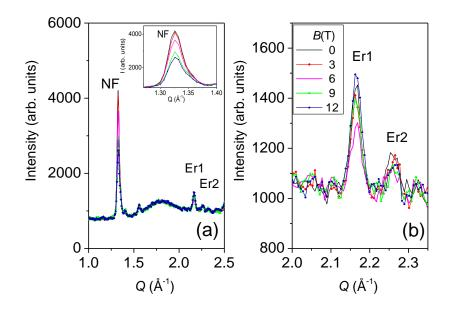
**Fig. 11.** Neutron powder diffraction patterns of  $Y_{0.5}Er_{0.5}Fe_2D_{4.2}$  recorded at 2 K under various magnetic fields on the E6 (BENSC) spectrometer ( $\lambda = 2.454$  Å). Inset (a) zoom on NF peak. (b) zoom on Er1 and Er2 peaks.
