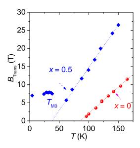
**Fig. 5**: Transition field  $B_{\text{Trans}}$  versus temperature for Y<sub>1-x</sub>Er<sub>x</sub>FeD<sub>4.2</sub> compounds (x=0, 0.5).
