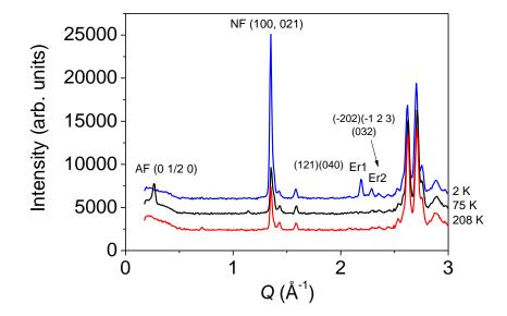
Fig. 8: NPD patterns of Y<sub>0.5</sub>Er<sub>0.5</sub>Fe<sub>2</sub>D<sub>4.2</sub> (sample S2) at *T*=2, 75 and 208 K measured on *D1B*  $(Q = 4\pi \sin\theta/\lambda; \lambda = 2.52 \text{ Å}).$
