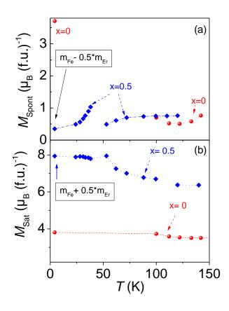
**Fig. 6**: Temperature evolution of the spontaneous magnetization  $M_{\text{Spont}}$  (a) and of the saturation magnetization  $M_{\text{Sat}}$  (b) for the Y<sub>1-x</sub>Er<sub>x</sub>FeD<sub>4.2</sub> deuterides (*x*=0, 0.5).
