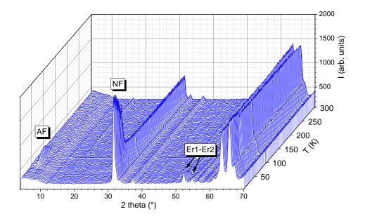
**Fig. 7**: Temperature evolution of the NPD patterns of  $Y_{0.5}Er_{0.5}Fe_2D_{4.2}$  (sample S2) recorded every 3 K between 2 and 300 K, as measured on the *D1B* diffractometer ( $\lambda$ = 2.52 Å).
