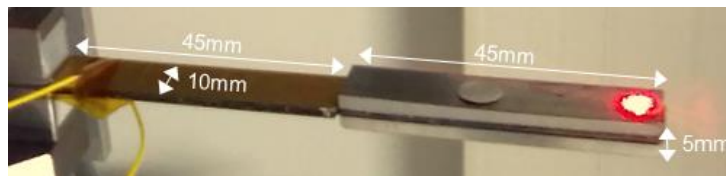
Figure 4. Fabricated prototype under test ( h_s=h_p=0.5\text{mm} )
