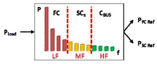
Fig. 5. Bandwidth splitting technique
