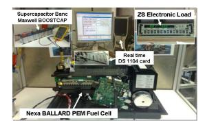
Fig. 11. Experimental bench components
