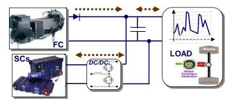
Fig. 3. One-converter parallel structure for FC/SCs hybrid power system.
