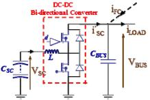
Fig. 7. Architecture of DC-DC Converter
