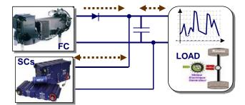
Fig. 2. Direct parallel structure for FC/SCs hybrid power system.
