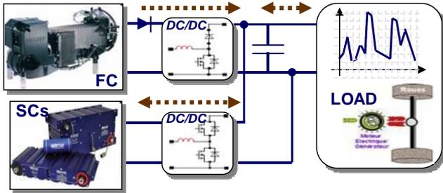
Fig. 1. Two-converter parallel structure for FC/SCs hybrid power system.
