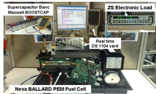
Fig. 11. Experimental bench components
