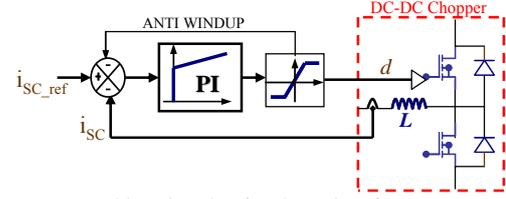
Fig. 8. Inner control loop insuring fast dynamics of SCs current
