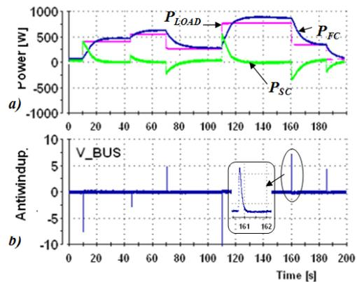
Fig. 14. Anti-windup output waveform of the voltage loop.
