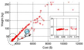
Fig. 7. Optimization results of the Weight/Cost objective functions.
