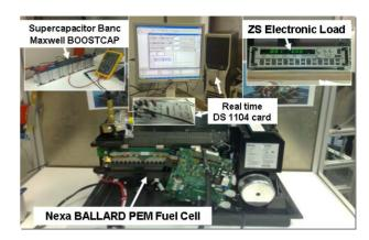
Fig. 5. The components of the experimental bench.
