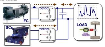
Fig. 1. Two-converter parallel structure for FC/UCs hybrid power system.
