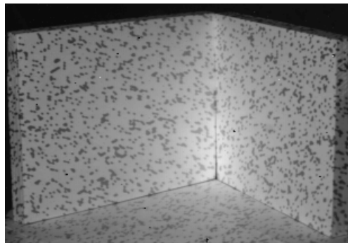
Figure 4: Random cloud projected onto two white planes. The black speckle is the projected IR light shadowed by the mask.
