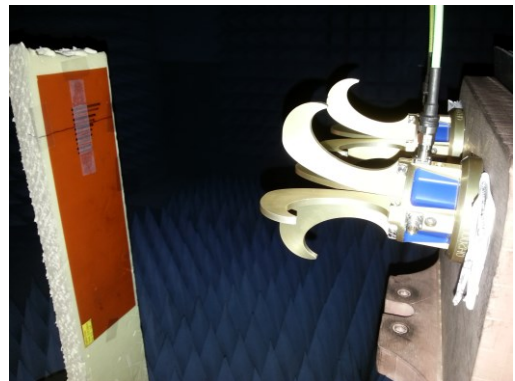
Fig. 5. Photograph of the tag applied on a Kapton film in the anechoic chamber.
