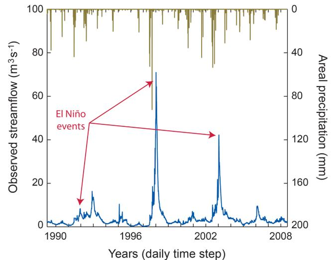
**Figure 2.** Interannual variability in precipitation and observed streamflow from 1989 to 2008. The hydrological year was defined from May to April so as to capture the snowmelt and peak flow seasons at mid-year (the graduations on the x axis indicate the 1 January of each year). Streamflow values are those measured at the catchment outlet before accounting for water abstractions. Precipitation values are those obtained after interpolation.
