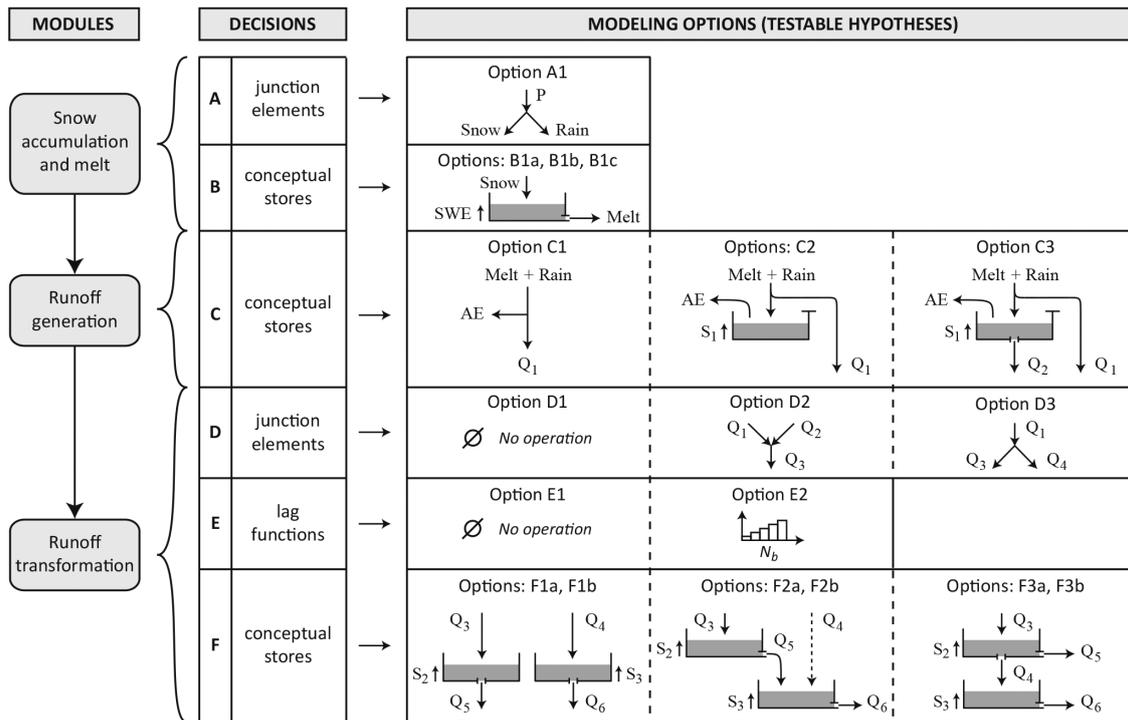
**Figure 3.** Overall architecture (modules), decision tree and available modelling options of the modular multiple-hypothesis framework (P: catchment-averaged daily precipitation; SWE: snow water equivalent; AE: catchment-averaged daily actual evapotranspiration;  $S_j \in [1, 5]$ : state variables of the conceptual stores;  $Q_j \in [1, 5]$ : water fluxes between the model components).
