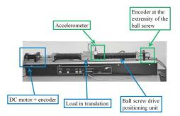
Fig. 1. EMPS prototype
