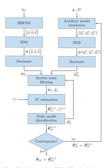
Fig. 3. Block diagram of the IDIM-AIV methodology
