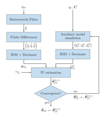
Fig. 2. Block diagram of the IDIM-IV methodology
