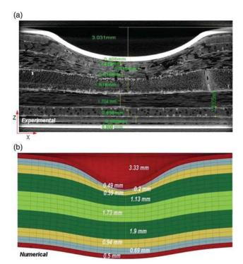
Figure 13. Comparison of plastic deformation and indentation for (plywood a/ aluminum skin) (a) experimental, (b) numerical.
