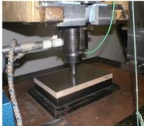
Figure 1. Drop-weight impact test set-up and aluminum wood specimen installed.
