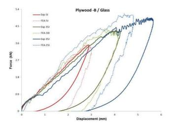
Figure 18. Force–displacement plot at 5 J, 1 0 J and 15 J (plywood B/ glass skins).
