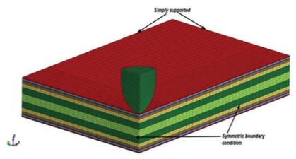
Figure 4. Numerical model for drop-weight impact.
