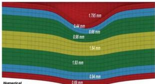
Figure 11. Comparison of crushing for plywood –A at 10 J (a) experimental, (b) numerical.
