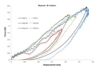
Figure 15. Force-displacement plot at 5 J, 10 J and 15 J (plywood – B/carbon skins).
