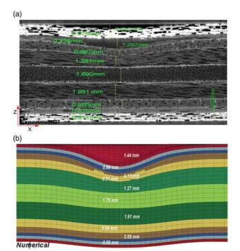
**Figure 19.** Comparison of plastic deformation and indentation for (plywood A/ glass skins) (a) experimental, (b) numerical.
