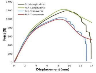
**Figure 8.** Force–displacement curve (plywood A/aluminum skins) - 3 point bending.
