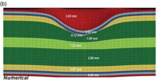
Figure 21. Comparison of plastic deformation and indentation for plywood – A/glass skins (a) experimental, (b) numerical.
