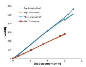
Figure 7. 3 point bending test on plywood A, force-displacement curve.
