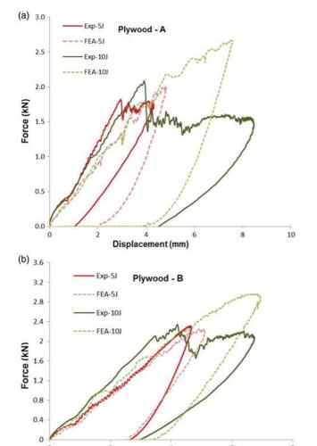
Figure 10. Force-displacement plot at 5 J, 10 J - (a) plywood A, (b) plywood B.
