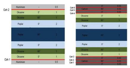
Figure 5. Cohesive element locations (red lines - color figure available online).
