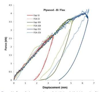
Figure 20. Force–displacement plot at 5 J, 10 J and 15 J (plywood – B/ flax skins).
