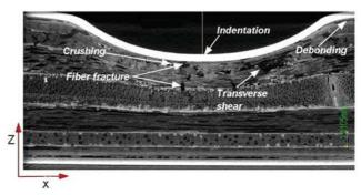
Figure 3. Tomography images of the center of impacted plywood with aluminum skin – Failure pattern at 15 J.
