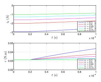
Fig. 6. Chronographs of  $i_d(t)$  and  $\tau(t)$  for  $\omega = 300$  rad.s<sup>-1</sup> and  $\tau_{ext} = 0$
