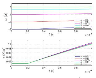
Fig. 5. Chronographs of  $i_d(t)$  and  $\tau(t)$  for  $\omega = 100 \text{ rad.s}^{-1}$  and  $\tau_{\text{ext}} = 0$ VI. CONCLUSION
