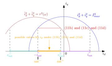
Fig. 4. Voltage and current limits (11b) and (11c) in  $(i_d, i_q)$ -plan
