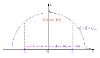
Fig. 2. Current limits (11b) in  $(i_d, i_q)$ -plan
