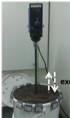
Lab-scale digestate tank
