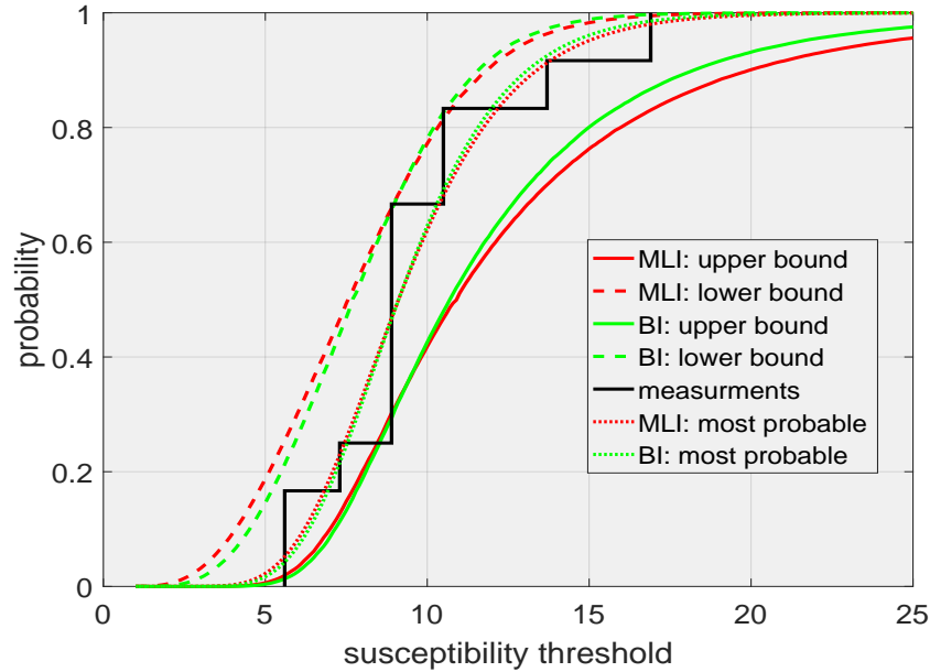
Figure 17. Family A estimated susceptibility thresholds distribution: empirical (black), most probable (from BI) (green small dot) and from MLI (red small dot) and bounds of confidence: upper bound with BI (green dot) , with MLI (red dot) and lower bound with BI (green), with MLI (red).
