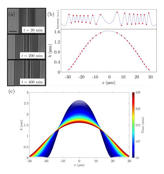
FIG. 2. (a) Typical optical microscopy images showing the temporal evolution of the interference fringes due to the liquid bump capped by the elastic plate (20  $\mu$ m scale bar). (b) Intensity profile averaged along the y-direction of the bump at a given time t, and corresponding reconstructed bump profile at 400 minutes. (c) Temporal evolution of the bump profile.
