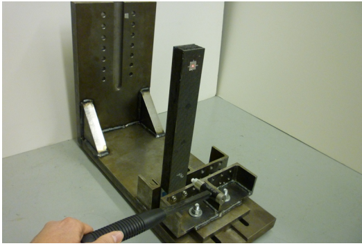
Figure 6: Experimental set-up for transient testing.
