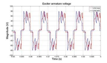
Fig. 2. Experimental (red) dq-model and simulated (blue) exciter armature voltage at nominal operating point ( $t_{sim} = 5 \text{ s}$ ,  $f_s = 100 \text{ kHz}$ ). (For interpretation of the references to colour in this figure legend, the reader is referred to the web version of this article.)
