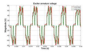
Fig. 12. Experimental (red) and Flux2D/Matlab simulated (green) exciter armature voltage at nominal operating point ( $t_{sim} = 0.1$  s,  $f_s = 100$  kHz). (For interpretation of the references to colour in this figure legend, the reader is referred to the web version of this article.)
