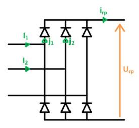
Fig. 7. Electrical equivalent circuit of the rectifier.
