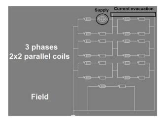
Fig. 4. Electrical circuit for identification purposes.
