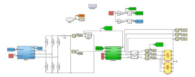
Fig. 1. Simulink dq-model of a self-excited alternator.
