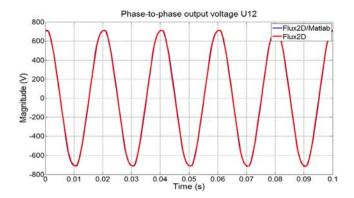
Fig. 10. Finite elements (red) and Flux2D/Matlab (blue) simulated main generator armature voltages  $U_{12}$  at nominal operating point ( $t_{sim} = 0.1$  s,  $f_s = 100$  kHz,  $U_{rp} = 22$  V). (For interpretation of the references to colour in this figure legend, the reader is referred to the web version of this article.)
