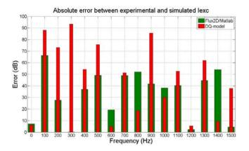
Fig. 17. Absolute error for exciter field current  $I_{exc}$  between experimental and Flux2D/Matlab results (green) and experimental and dq-model (red). (For interpretation of the references to colour in this figure legend, the reader is referred to the web version of this article.)
