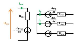
Fig. 6. Electrical equivalent circuit of the exciter.
