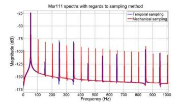
**Fig. 5.** Spectra of the mutual inductance between rotor and stator phase 111 sampled with mechanical  $(1^{\circ}, \text{red})$  and temporal (0.1 ms, blue) steps. (For interpretation of the references to colour in this figure legend, the reader is referred to the web version of this article.)
