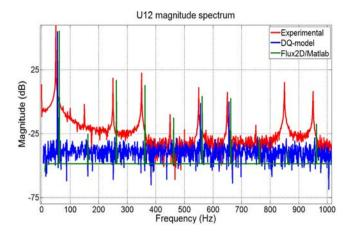
Fig. 16. Spectral contents of experimental, dq- and Flux2D/Matlab-simulated main generator armature voltages  $U_{12}$  ( $t_{sim} = 1$  s,  $f_s = 100$  kHz, artificial shifting).
