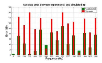
Fig. 19. Absolute error for alternator field current  $I_{rp}$  between experimental and Flux2D/Matlab results (green) and experimental and dq-model (red). (For interpretation of the references to colour in this figure legend, the reader is referred to the web version of this article.)
