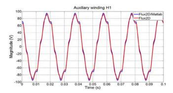
Fig. 11. Finite elements (red) and Flux2D/Matlab (blue) simulated auxiliary winding H1 electromotive force at nominal operating point (tsim = 0.1 s, fs = 100 kHz, Urp = 22 V). (For interpretation of the references to colour in this figure legend, the reader is referred to the web version of this article.)
