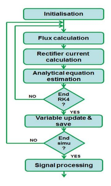
Fig. 9. Algorithm for analytical equations identification.
