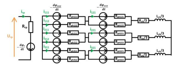
Fig. 8. Electrical equivalent circuit of the alternator.
