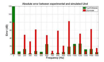
Fig. 18. Absolute error for exciter voltage  $U_{ind}$  between experimental and Flux2D/Matlab results (green) and experimental and dq-model (red). (For interpretation of the references to colour in this figure legend, the reader is referred to the web version of this article.)
