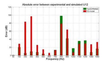
Fig. 20. Absolute error for alternator voltage  $U_{12}$  between experimental and Flux2D/Matlab results (green) and experimental and dq-model (red). (For interpretation of the references to colour in this figure legend, the reader is referred to the web version of this article.)
