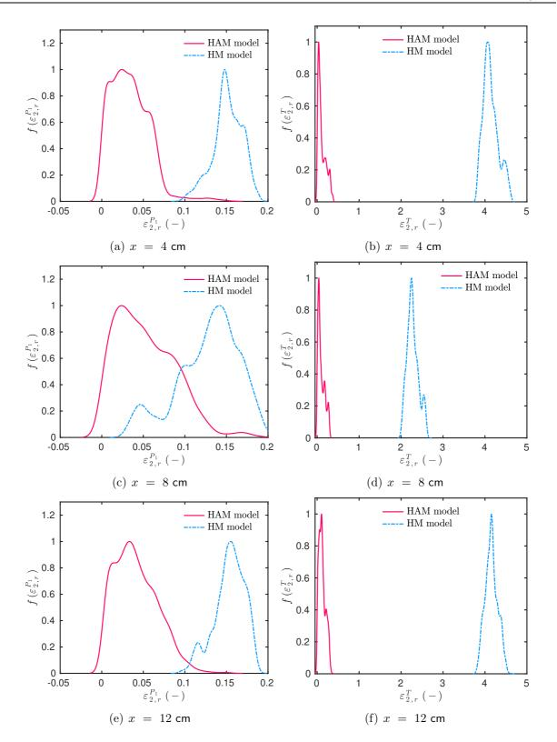
**Figure 12.** Comparison of the probability density function of the relative error between the experimental observations and the numerical predictions for vapor pressure (a,c,e) and temperature (b,d,f), obtained with the proposed model and the purely diffusive one.
