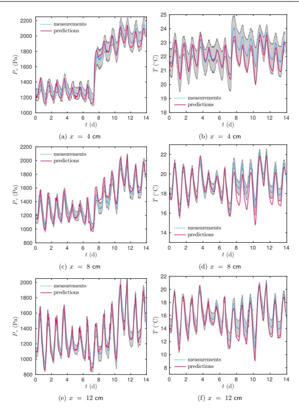
**Figure 8.** Comparison of the experimental observations with the numerical predictions for vapor pressure (a, c, e) and temperature (b, d, f). The grey shadows represent the measurement uncertainties.
