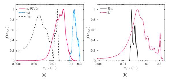
**Figure 6.** Probability density function of the relative error for some hypothesis in the formulation of the mathematical model (a) for the latent heat of vaporization  $r_{12}$ , for the volumetric heat capacity  $c_q$  and for the transient term in the right hand side of the heat Equation (2.14b) and (b) for the for the constant gas law  $R_{13}$  and the gradient of enthalpy.
