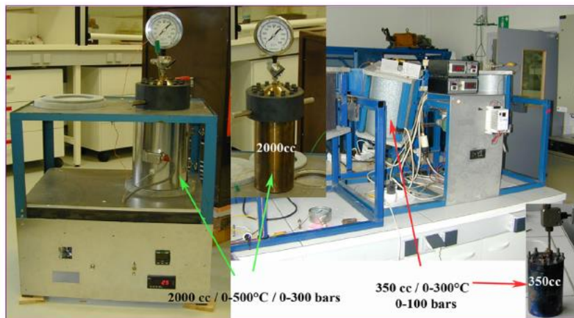
Fig. 2. Different batch type reactors from 350 to 2000 cc for temperatures ranging from 0 to 500 °C and maximum pressures of 300 bar.
