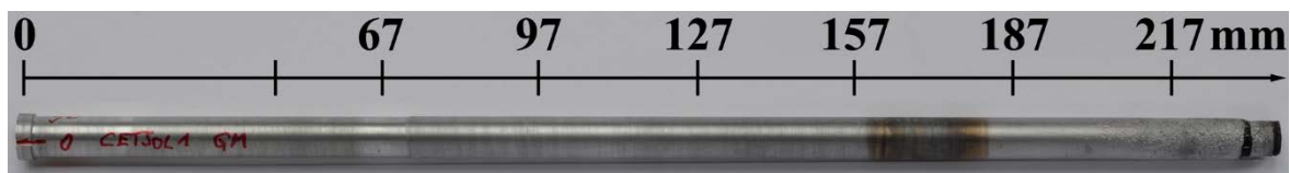
Fig.2. Photograph of the processed GM sample with identification of cross-section positions.
