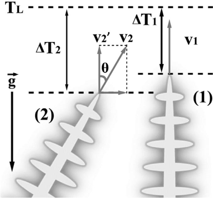
Fig.9. Schematic tip growth velocity of two dendrites with different orientations relatively to the temperature gradient direction: (1)  $0^\circ$  and (2)  $\theta$ . The upper dash line indicates the liquidus isotherm position ( $T_L$ ).  $\Delta T_1$  and  $\Delta T_2$ , and  $v_1$  and  $v_2$  are the tip undercooling and growth velocities of dendrites (1) and (2), respectively.
