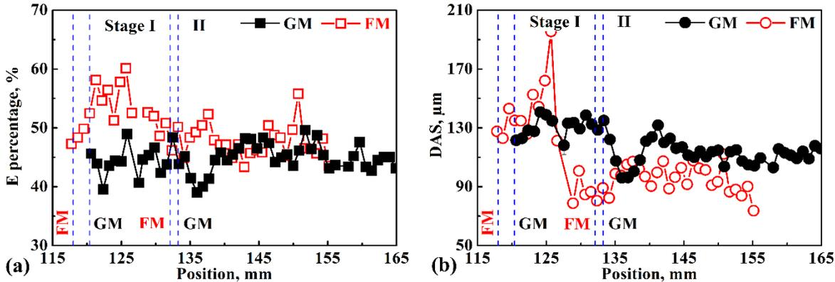
Fig.5. (a) Mean eutectic percentage and (b) mean DAS vs. position along the longitudinal direction of both the GM and the FM samples. The boundaries between different
