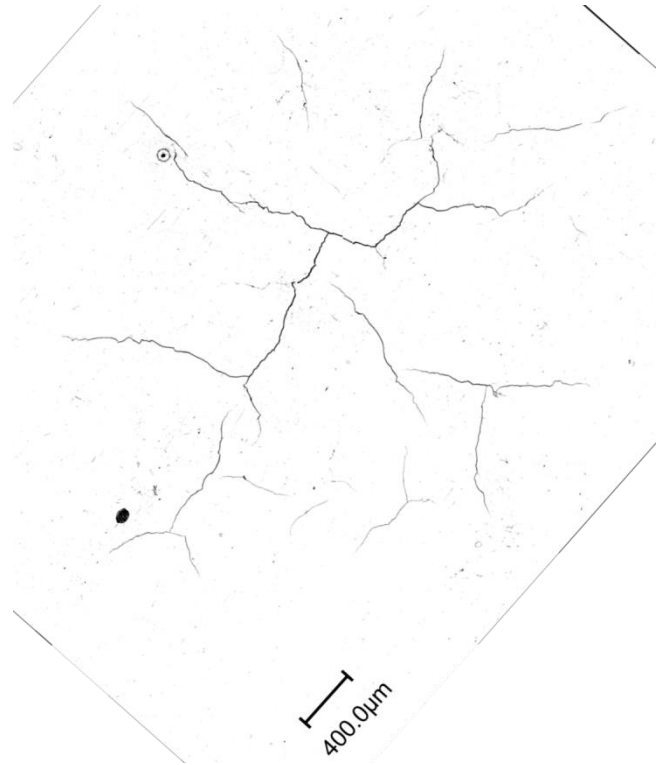
Fig. 8 Optical micrograph of crack network of K46T8-22 specimen when \Delta T = 230^{\circ}\text{C} coupled with a static mean tensile stress \sigma_b = 15 \text{ MPa} after 21,600 cycles
