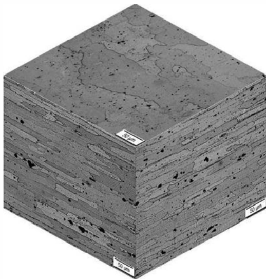
Fig. 7. Optical microscopic 3D views of the AA 7175T7351 substrate after degreasing and metallographic attack [55].
