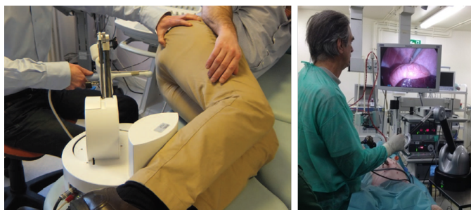
Figure 1. Comanipulating an instrument through a fulcrum: left – the 6-DOFs robot Apollo assists a urologist who manipulates an endorectal ultrasound probe to perform prostate biopsies [9]; right – the same concept applied to endoscopic surgery
