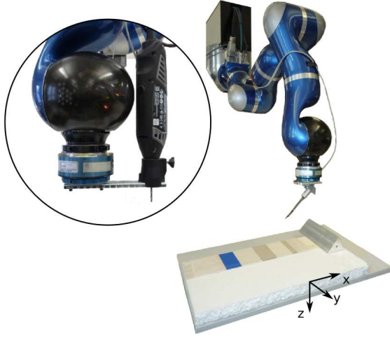
Fig. 4. Setup of experiments described in Section V with the DLR lightweight robot (LWR), the Dremel drill attached to the robot end-effector in the zoomed end-effector and the scalpel in the main panel.
