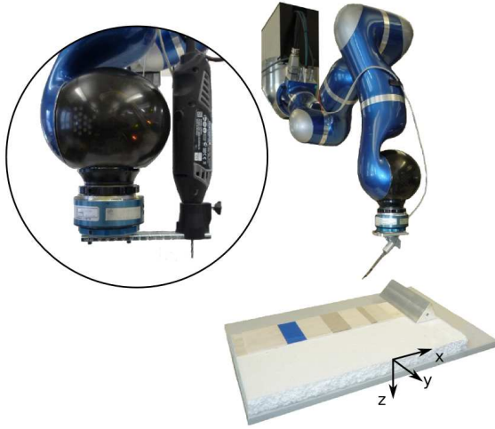
Fig. 4. Setup of experiments described in Section V with the DLR lightweight robot (LWR), the Dremel driller attached to the robot end-effector in the zoomed end-effector and the scalpel in the main panel.
