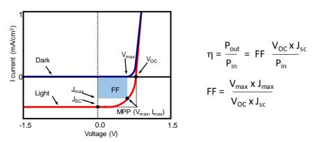
Figure 18. I/V curve of a PV device and characteristic values associated.
