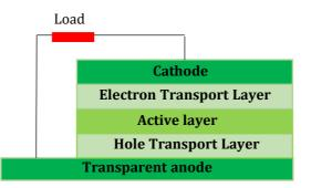
Figure 17. Structure of a bulk heterojunction OPV device.
