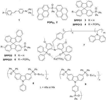
Figure 3. Phosphine materials as charge-transport and injection layers.
