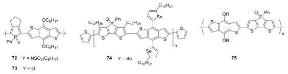
Figure 22. Phosphole containing polymers used for OSC devices.
