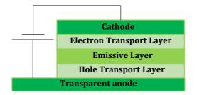
Figure 2. OLED structure.
