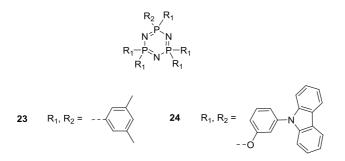
Figure 8. Phosphazene derivatives used in OLEDs.
