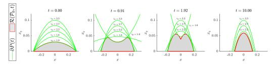
Figure 5: Time-varying paraboloids overapproximate the reachable set at different time instants t in  $\{0.00, 0.91, 1.62, 10.00\}$  for different initial conditions  $P_i(0) = \gamma_i \mathcal{P}_0$ , where scaling factors  $\gamma_i$  are respectively equal to 1.0, 1.6, 2.2, 2.7 and 3.3 for  $i = 0, \ldots, 4$ . The shaded regions are the reachable set  $\mathcal{R}(\mathcal{P}_0, t)$ , the thin green lines are the boundary of the overapproximation P(t) of Theorem 1.
